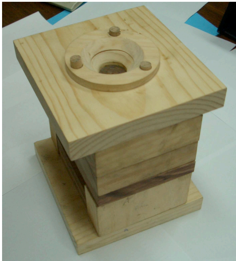
Figure 10. 3D timber mould model for producing a cup shaped product. Mould closed.
