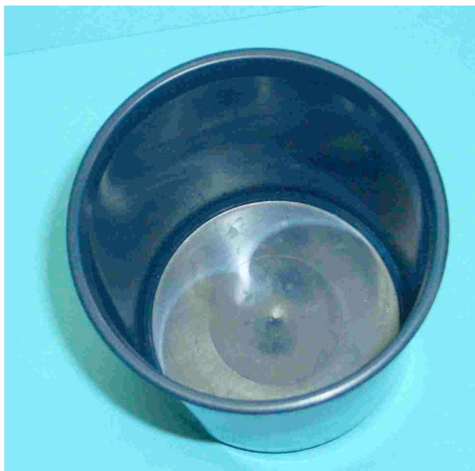
Figure 9. Cup-shaped moulded part. Ejector pin and gate can be observed in the image.
