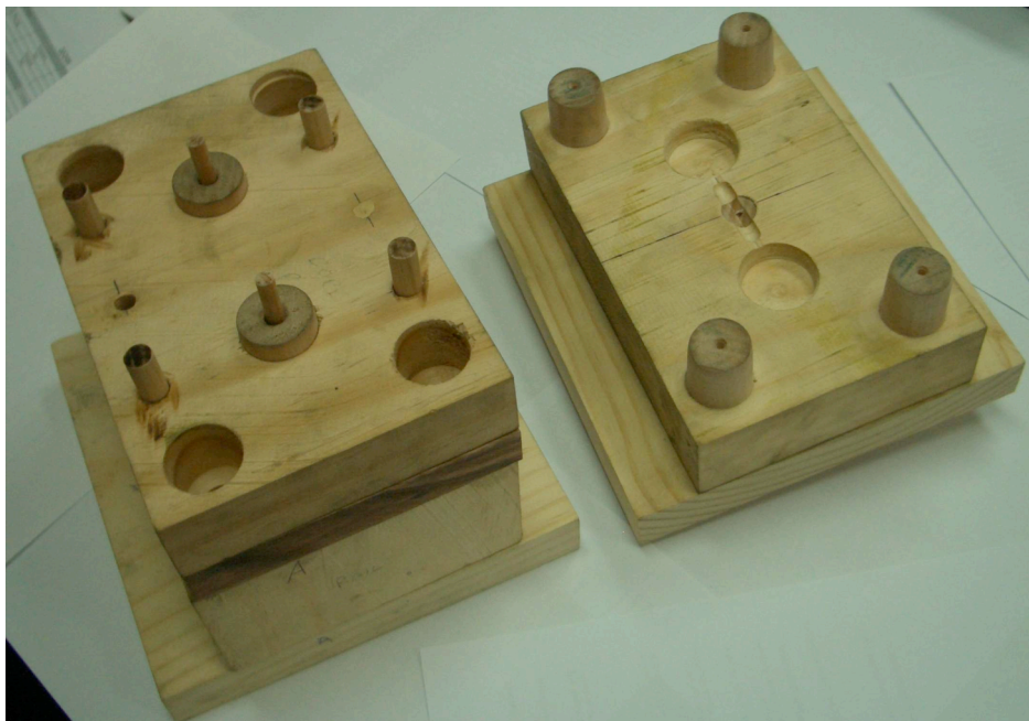
Figure 11. 3D timber mould halves, showing the ejection system activated
