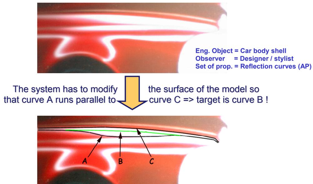
Figure 7. Shape Modification by Defining/Specifying Target Reflection Curves
