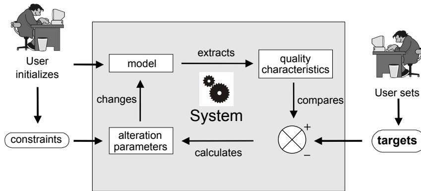
Figure 3. Principle of Engineering in Reverse (EiR) and Target Driven Design
