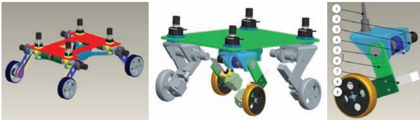
Figure 11. a) Chassis, b) alternative chassis, c) driving module of the mobile robot MAX 3D
