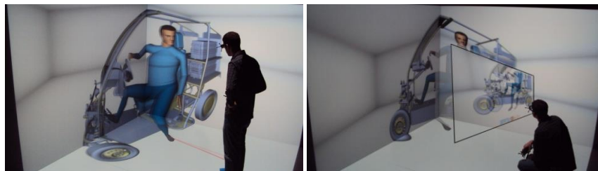
Figure 4. The ergonomist visualizes the vehicle with the virtual human (left). The ergonomist takes a snapshot to his viewpoint (right).
