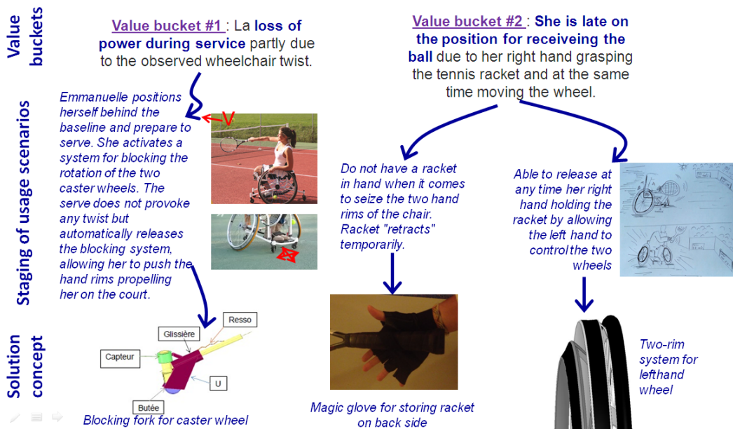
Figure 7. Illustration of the two-stage ideation process (scenario creativity and concept creativity) starting from the two value buckets identified for the handitennis wheelchair
