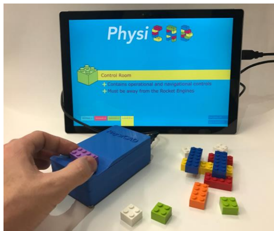
Figure 1. InstructiBlocks, a PhysiCAD system using RFID to embed design rules in LEGO bricks
